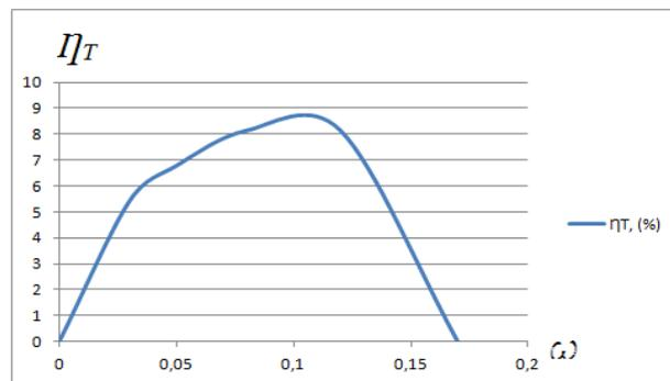
Fig.15. The characteristic curve of the turbine utilization factor  $\eta_T$ , depending on rpm
