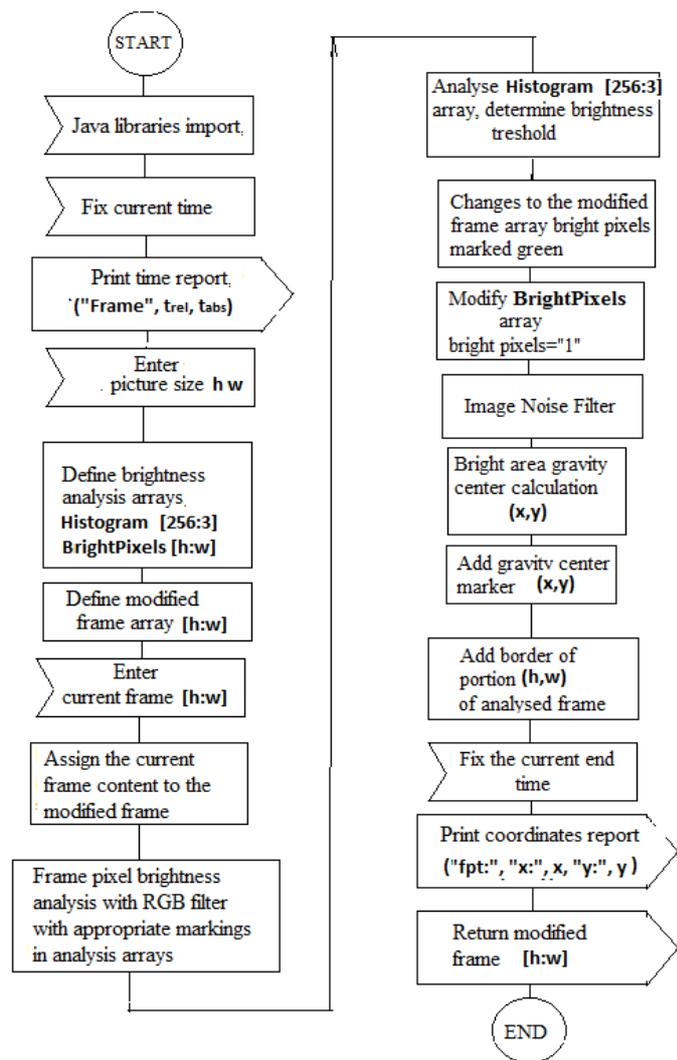
Fig. 7 Description of the structure diagram and language of the laser beam coordinate image processing program
