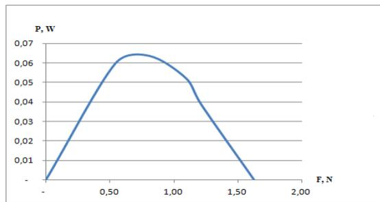
Fig. 14 Turbine power  $P$  (W) calculation results at different loads
