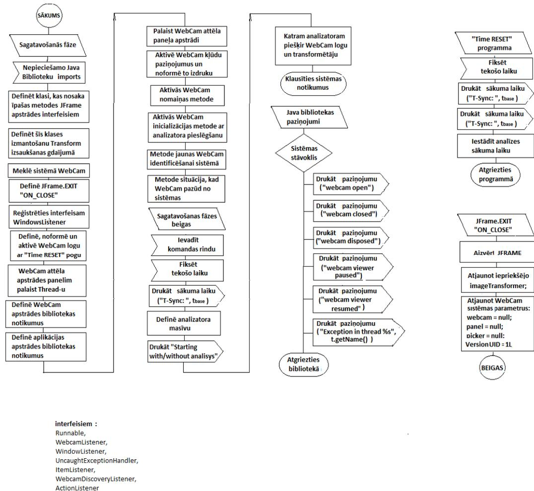
Fig. 8 Description of the structure and language of the WEB-camera image data capture program
