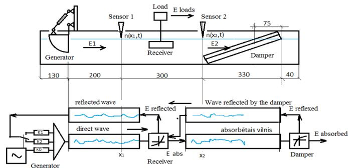
Fig. 11 Wave process analysis scheme [1]
