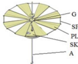
Fig. 10 *APRLHK* turbine construction (*G* - bearing, *SP* - tensioning rubber, *SAB* - self-adjusting blade, *SK* - pulley, *A*-axis)
