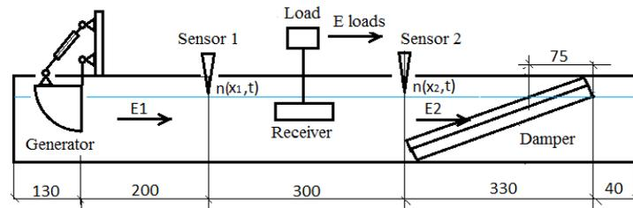
Fig.1. Principal Scheme of laboratory components [1]
