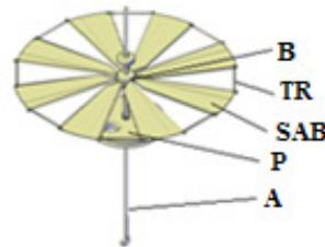
Fig. 3. ASRBHK turbine construction (B – bearing, TR – tensioning rubber, SAB – self-adjusting blade (SAB), P – pulley, A –axis) [29].
