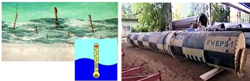
1p.31. att. Float Wave Electric Power Station – FWEPS [110]
